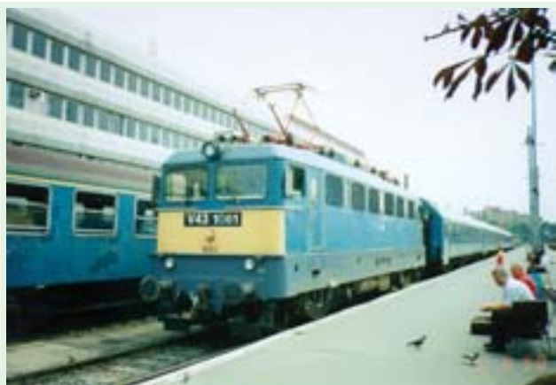
Electric traction provides high starting torque and low maintenance costs making it the best choice for trains
