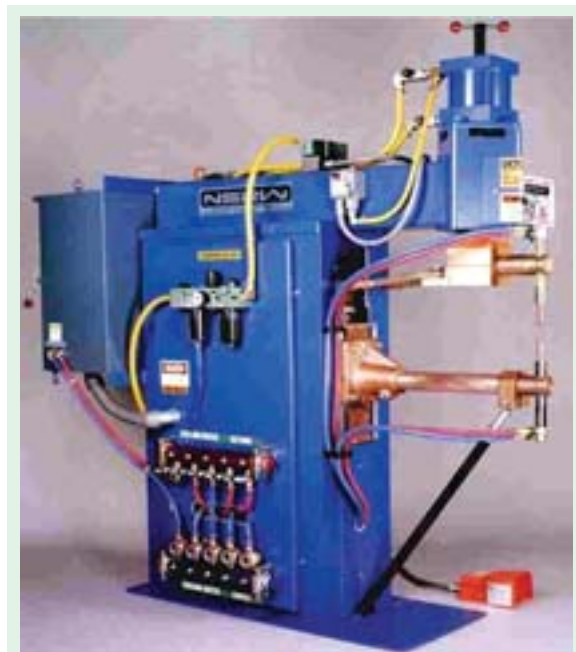
Spot welding machine
