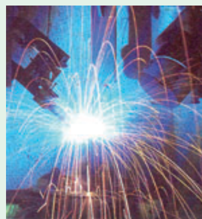
An electric arc is produced when electricity is passed between two electrodes
