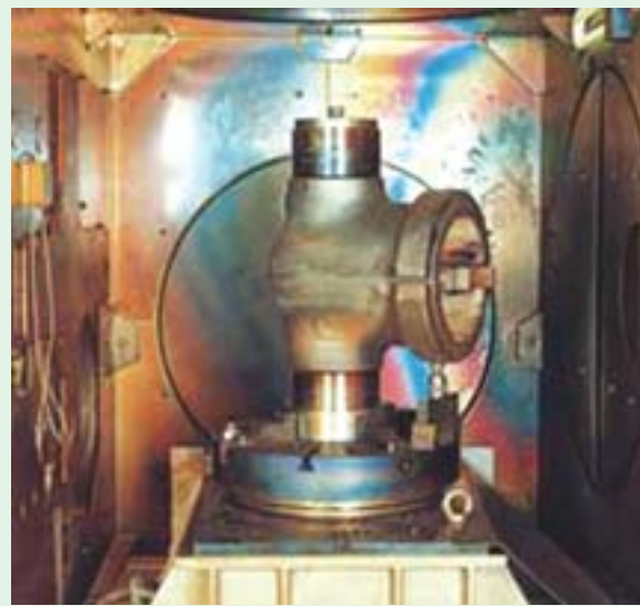
Electron beam welding facility
